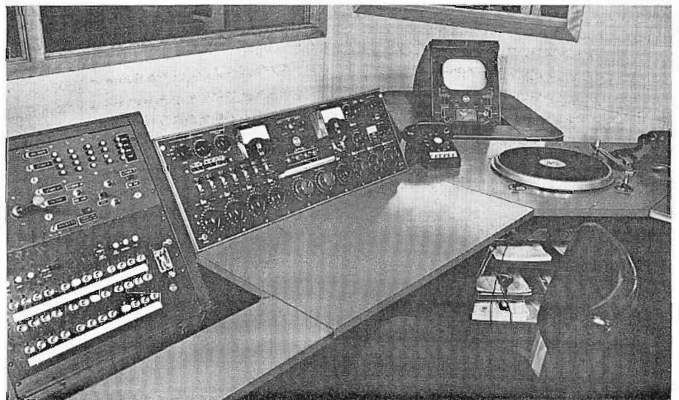
FIG. 10. Tv control showing a close up of the second TS-21 switching panel which is adjacent to the BC-6 audio console.
