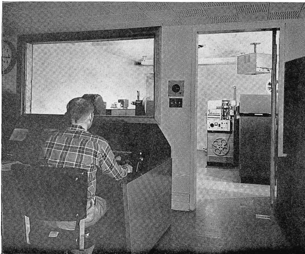
FIG. 12. Looking into the tv projection from the control room. Two projection equipment groups are included; one for standby use.
