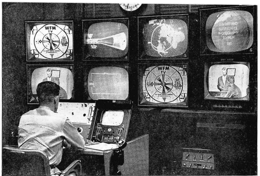
FIG. 25. Master control console, where pictures are selected for transmission on each of WFM-TV's seven channels.
