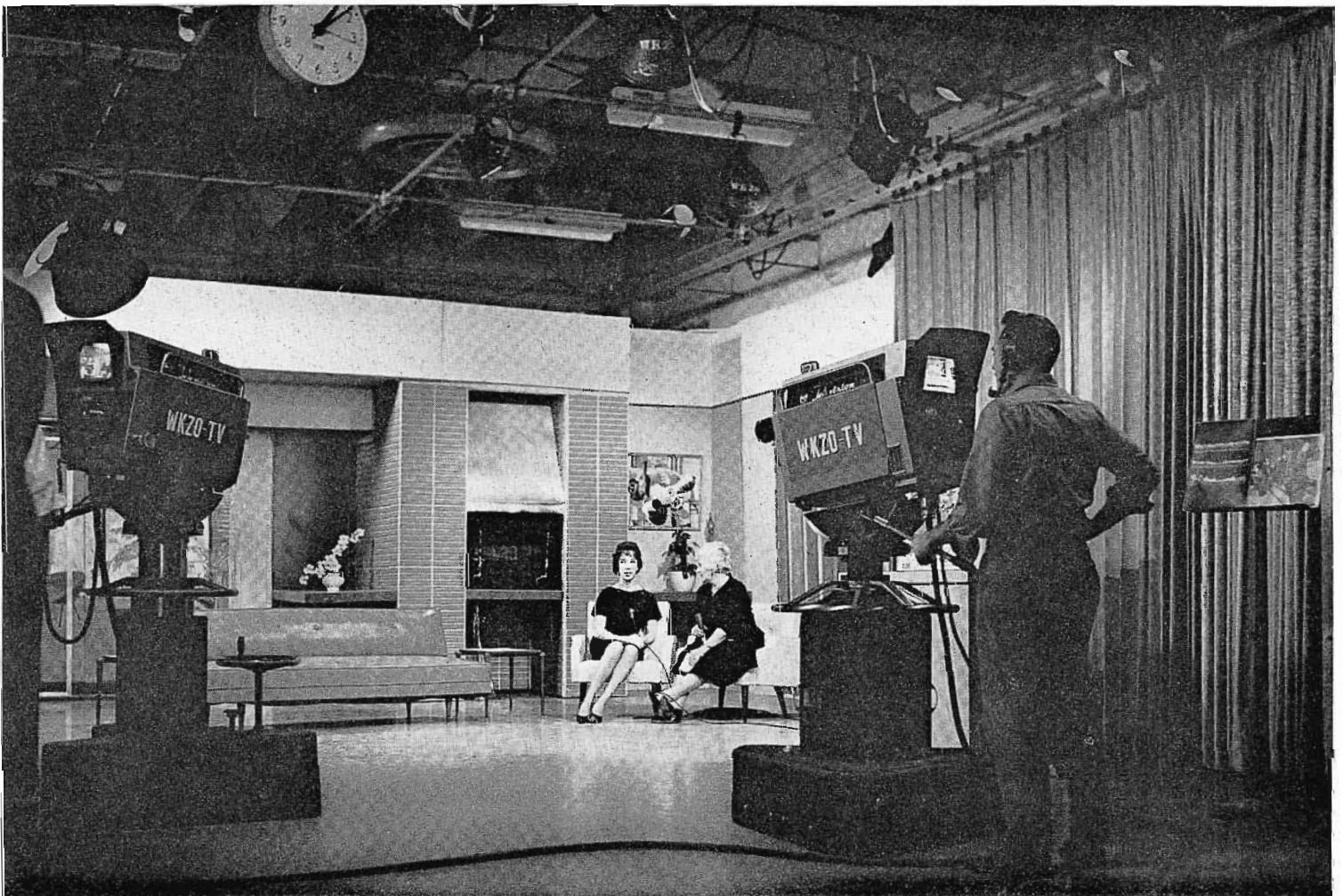
FIG. 7. "Studio 3" in use on Feminine Fancies women's show. Studio equipment includes two new TK-12 4½-inch image orthicon cameras.
