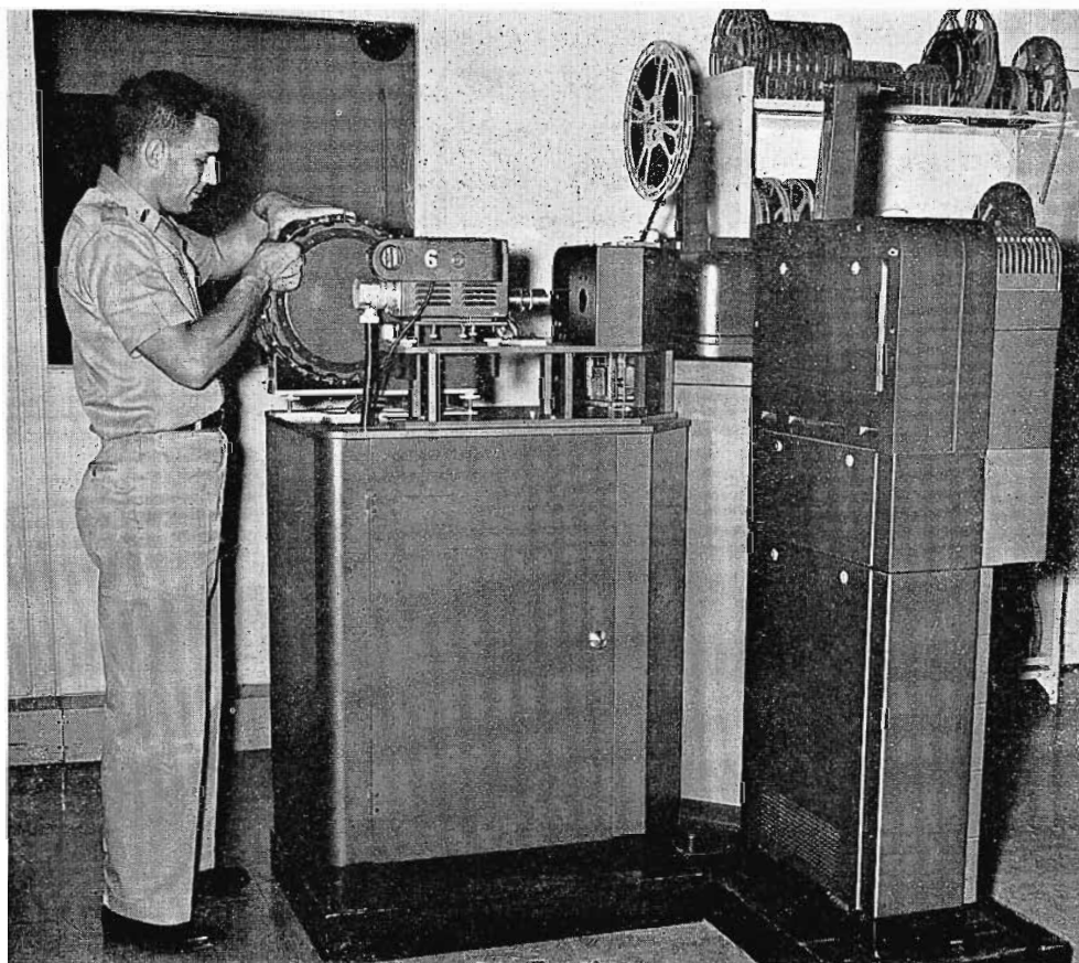
FIG. 24. CWO Darwin A. Koppie, Chief Engineer of TV Division re-loads the TP-7A slide projector.
